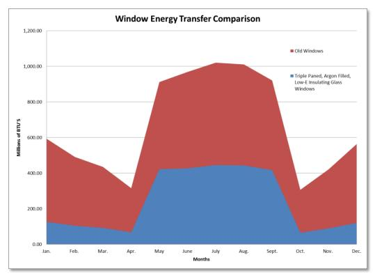
Figure 28. Window Energy Comparison
