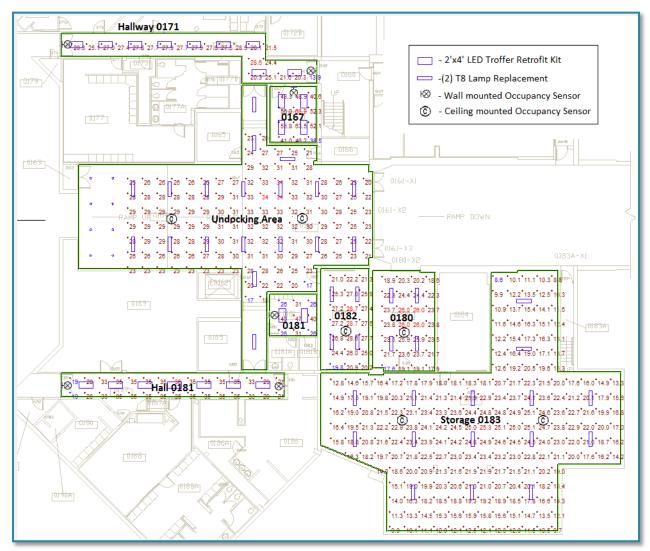
Figure 7. Proposed Lower Level Reflected Ceiling Plan
