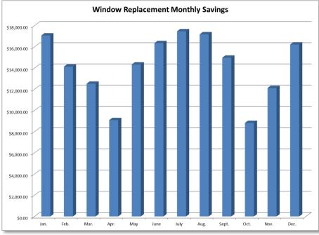
Bv calculating kWhs difference in between the existing and proposed windows with a minimum cost of energy at \$0.25 cents a kWh, there is а substantial vearly savings, as shown in Figure 30. With this data, we were able to find material costs and conduct a return on investment analysis, the results of which are in Table 11. From the payback provided by the energy cost savings these windows, for there will be a payback in 21.03 years.
